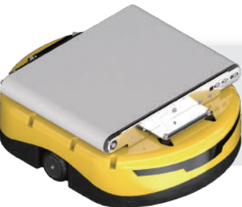
LBCRB20, cross belt sorting robot Dimensions (L*W*H) (mm) 480*380*200
