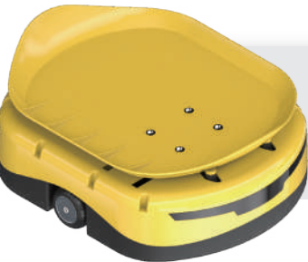
JTRobotII-2, standard model sorting robot Dimensions (L*W*H) (mm) 480*380*200
