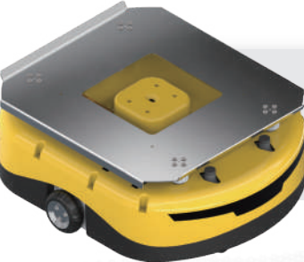
T-sort with lift Dimensions (L*W*H) (mm) 480*405*176
